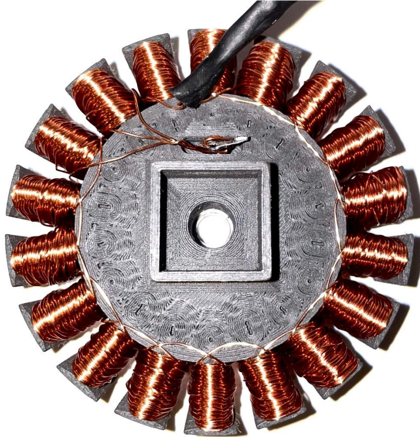
Figure 4: Winding Orientation and Final Configuration
